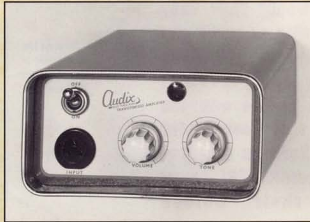
▲ An early 30watt transistorised amplifier made at the Stansted works.
