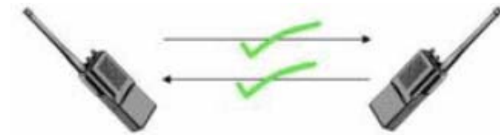
A simple illustration of a full-duplex communication system.
